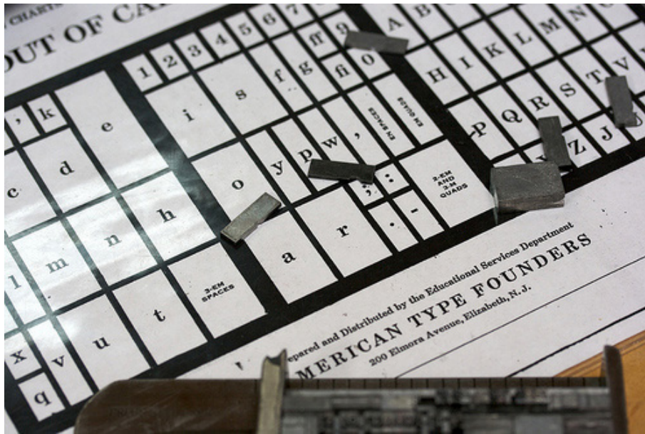
A chart displaying the layout of the California Job Case method for arranging type.
