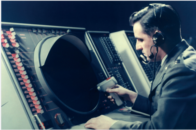
A SAGE controller selecting items on screen in 1958. (Used by kind permission of The MITRE Corporation.)
