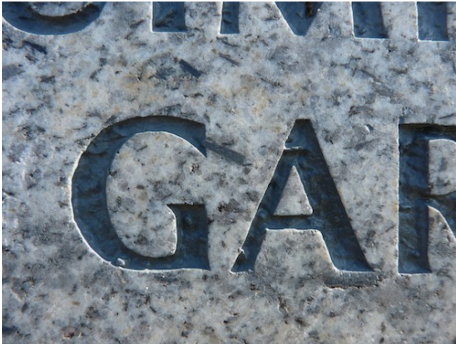
An example of an uppercase “G” and “A” carved in granite and infilled. The letters are sharp.
