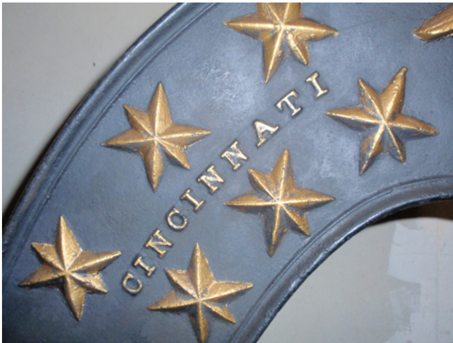
Cincinnati Type Foundry's acorn-shaped Press was made after the design of Stansbury, sometime between 1825 and 1856. The stars are a nice touch. The lettering is also Clarendon and quite regular, suggesting that punches were used to make the mould.
