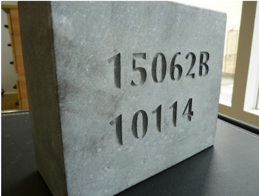
A piece of limestone was carved by hand and by laser to test the quality of the carving.
