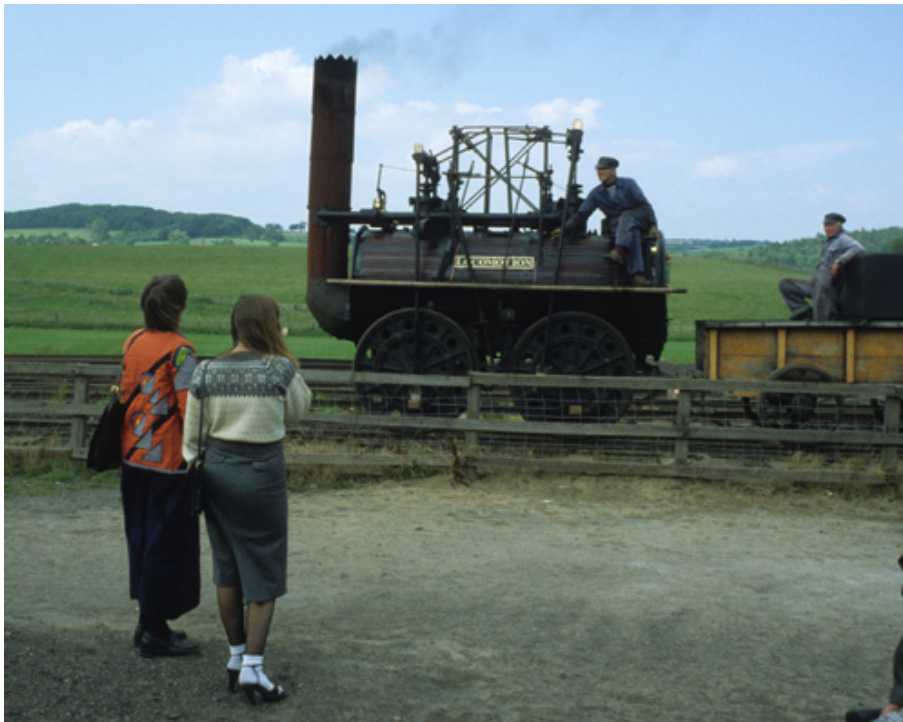
A replica of “Puffing Billy,” a giant boiler on wheels with a beam engine, runs at the Beamish Open Air Museum in County Durham, UK. Its nameplate reads “Locomotion” in sans serif.
