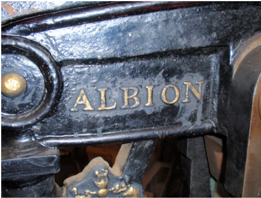
The Albion Press was another popular cast-iron printing press. The lettering is a stout modern face with bracketed serifs; in essence, a Clarendon. This one was made by Henry Watts of London in 1853.
